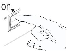
To turn the amplifier 'on', push in on the top portion of the rocker switch firmly. It should move inward and snap into the 'on' position. After switching on, the power LED should illuminate.
